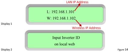
A word about network communication protocols: The ECU needs to have access to the router via a LAN IP address. The ECU will only search for and obtain a Dynamic Host Configuration Protocol (DHCP) IP address during its powering up sequence.
