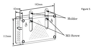
• Attach the ECU to the mounting rail with machine screws.
